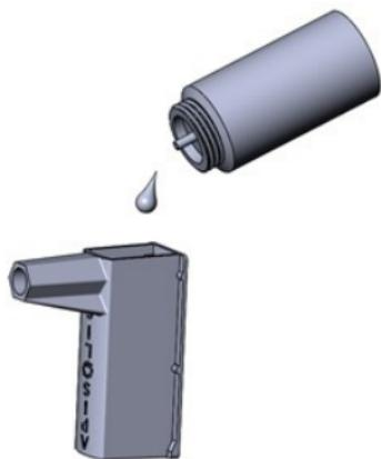
Pour the Native solution into the tank through the opening provided for this purpose. Warning: fill up to the limit of the internal reinforcements of the tank (see below).
